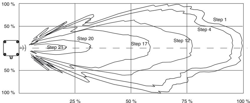
**Sensitivity adjustment for suppression of disturbing targets**
